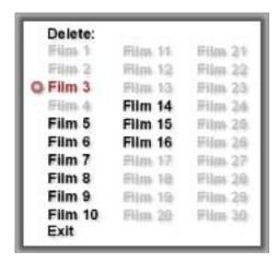
The Delete Menu allows you to delete existing videos from the banks. Select the respective storage bank and then press the **Ok** key. Additionally, the text `**Remove Video?**′ must be confirmed with `**Yes**′.
